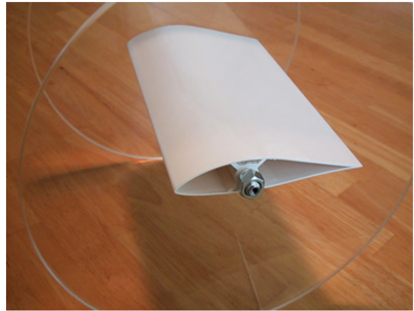
Stereo-lithography used to develop the Wortmann FX-S-02-196 Airfoil
