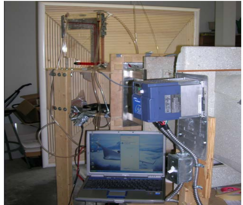
Experimental set-up showing the pressure transducers and manometer
